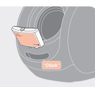
Insert the cartridge Open the slot, romove the cover cap on the cartridge and insert. Push in the cartridge completely until you hear a clicking sound.
