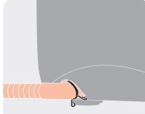
Connect the drain hose Connect the drain hose to the outlet, and secure with the clamp.
