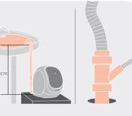
The inbuilt drain pump can pump water vertically as high as 70cm above the floor. Connect the drain hose to a floor drain, drain pipe or a sink. Use the Y-piece if necessary.
