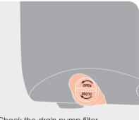
Check the drain pump filter Make sure the filter is tightened. (The word 'OPEN' should face up) \* Clean the filter every month.
